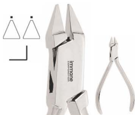
Article# IC8-073 Adams Plier Adams pliers for bending wire arches and bends right angles for wires up to .022", .025 tip to beak. Length 13cm
